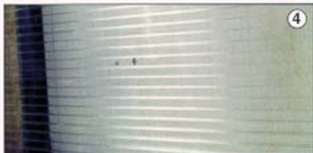
QuickGuard® Polycarbonate Panel After Impact No Failure
